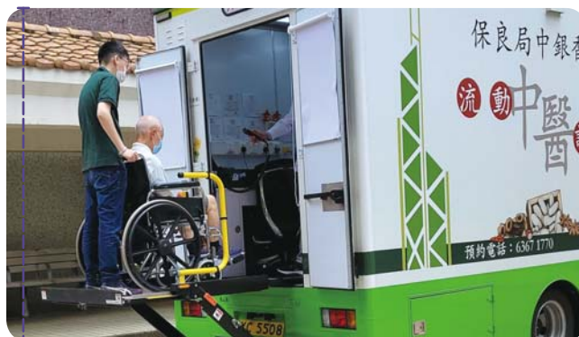
本局的流動中醫診所設有升降台，方便行動不便人士診症。 Our Chinese Medicine Mobile Clinic was equipped with a lifting platform to facilitate consultation for people with mobility difficulties.
